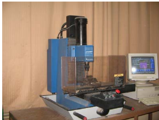
(a) ProLight2000 CNC end milling machine
