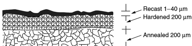
Fig. 2. EDM heat affected zone (El-Hofy, 2005).
