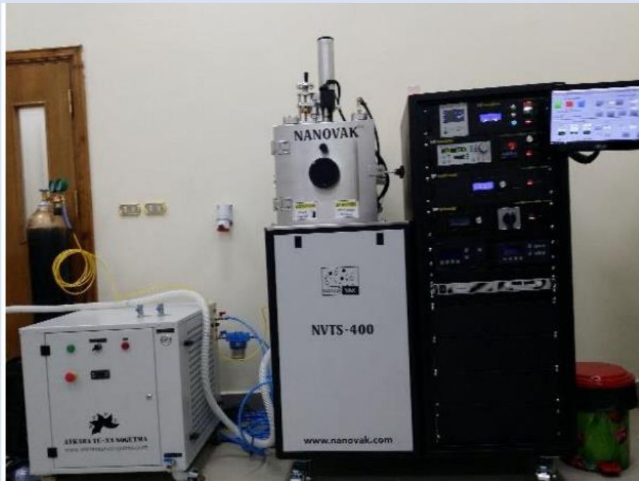
Figure 2-22. photographic image and Schematic drawing of thermal evaporator.
