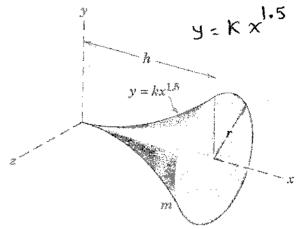
2. (b) (10 Marks) Calculate the moment of inertia of the shaded area about x-axis and y-axis.
