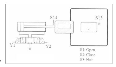
by solenoid valve Y1 after a delay of 6 seconds. The closing procedure can also be commenced by means of button S2. Stop button S3 can be used to halt the closing of the door. If a total opening time of 30 seconds is exceeded through repeated operation of the stop button, this button is disabled and the furnace door closes automatically. Closing of the door is completed by deactivating solenoid valve Y1 when limit switch S13 is reached.
